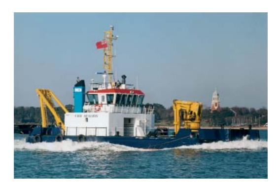
UKD Sealion is a 25 metre Multicat built by Damen Shipyards for UK Dredging. She is specified to provide a multi purpose dredging support vessel with bed levelling, buoy handling and survey capability. Her principal duties are those of a bed leveller and her 10 metre plough is capable of working at a depth of 20 metres.
