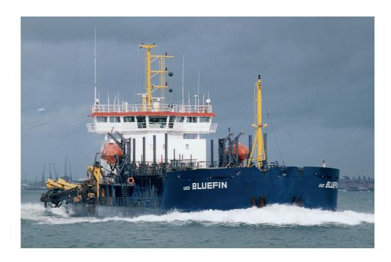
UKD Bluefin is a purpose-designed trailing suction hopper dredger with many advanced features. Special attention has been paid to hull form and dredge-gear layout to enable this vessel to dredge in open-sea conditions while maintaining efficiency. She is fitted with twin suction pipes and pumps, jet pumps and de-gassing gear; underwater overflow is via an adjustable weir and she has the ability to discharge via bottom doors or pump ashore.
