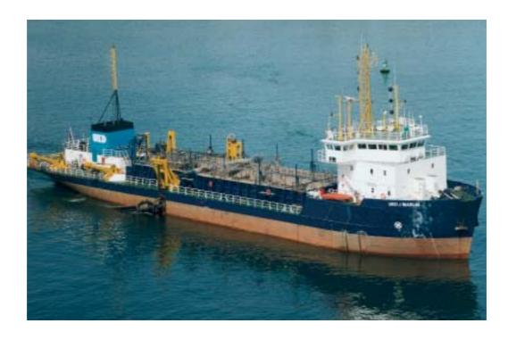
A modern trailing suction hopper dredger designed for use in open sea and estuarial locations, UKD Marlin has the ability and manoeuvrability to dredge in confined locations such as enclosed docks. The vessel is equipped with twin suction pipes, swell compensators, de-gassing and drag-head jets. She has the facility to discharge via bottom doors or to pump ashore and is fitted with an underwater overflow via an adjustable weir.
